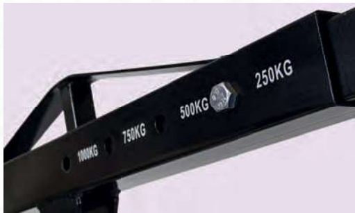
4 hole position boom with indicated weight capacities
